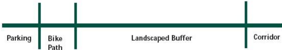
Figure 7: Example of how the extension of the Barnegat Branch Trail within the former rail ROW can be integrated along Route 166.
